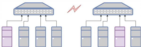
This situation is known as **split brain**; a condition where two sides are not able to communicate but continue to work independently. The problem is what happens when the link is reconnected – you end up with two masters, two copies of all data and VMs that may have diverging contents.
