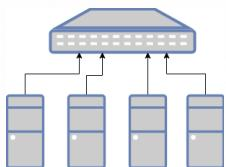
With all the nodes connected to a single switch. If a node fails, the others are unable to reach its internal IP address, and the system decides after a predetermined period to mark it as "dead" and the data and VM that were hosted there are recreated on another available node. Now, let's imagine a more complex scenario:
