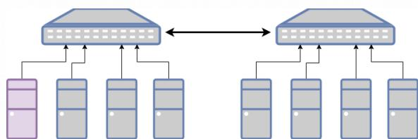
We have now two switches, with an uplink between the two (the purple node is the master). Let's imagine that the uplink fails, so that we end up with two separate networks; in this condition, the second network is unable to reach the old master (and the other 3 nodes) and will thus miss a master. This will force a new election, and each network partition will assume the other nodes disappeared, forcing a replication of all the data and VMs that were on the other side:
