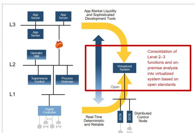
This approach leaves to physical platforms only the small number of L1 control systems that require hard real-time or strict latency properties, while consolidating the remaining infrastructure into a single Edge cloud platform that provides flexibility and hardware independence.
